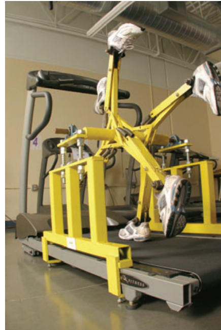
One of the many tools we use to test treadmill life
